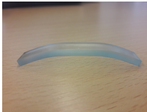
Figure 4.4: Photograph of the a highly deformed epoxy resin specimen after a stress relaxation test.
